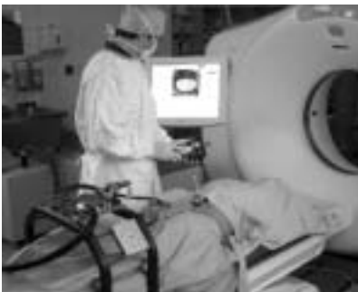
Set-up for a CT-guided robot-assisted biopsy procedure of the new prototype B-ROB II developed by Kronreif et al.
